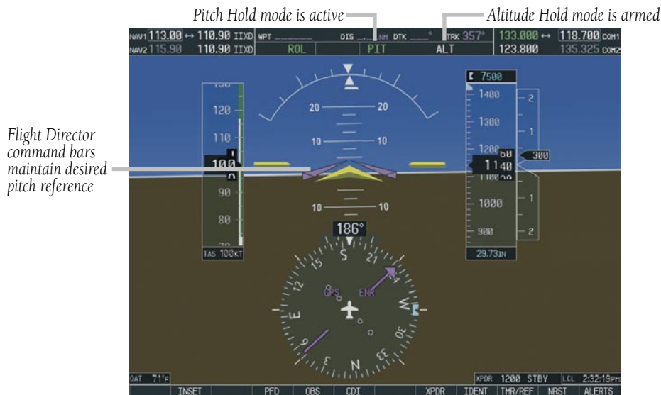
Figure 6-10 Pitch Hold Mode
